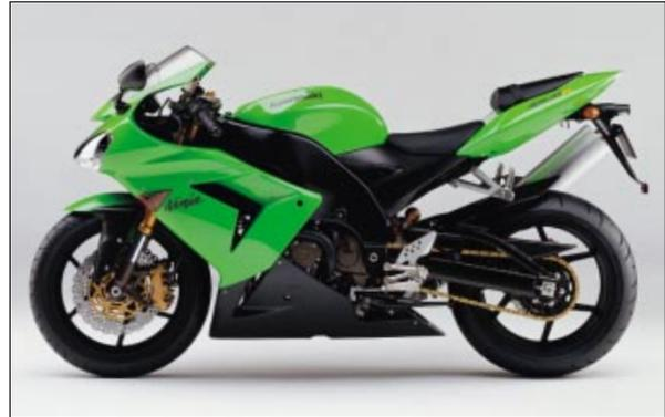
Unlike most other Kawasaki machines, the Ninja ZX-10R design started with chassis simulations. The engineers wanted an extremely lightweight and compact chassis that would offer superb handling and stability. The combination of a short wheelbase with a long swingarm is a configuration also seen on the Ninja ZX-RR. An all-aluminium frame with 600-class dimensions mated to a long and highly rigid gull swingarm gives the ZX-10R category-leading handling performance on track and twisty roads.
